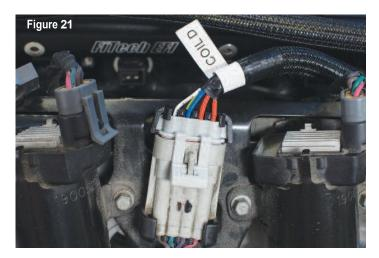
**Coil D:** The Coil D connector is connected to the existing connector on the driver's side coil pack. **Note:** Coils and coil sub harnesses are not included in
