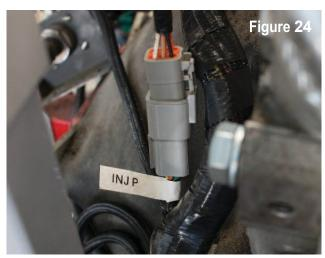
**Injector P/Injector D:** (Passenger side connector shown): Each of these connectors mate with the included injector sub-harness on the for each side of the intake manifold.
