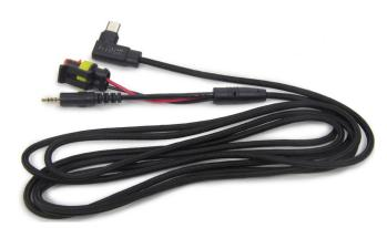
Handheld Controller Cable: Connects the ECU to the Handheld. The 2-wire connection on the harness supplies constant battery 12 Volts and ground to the Handheld. The stereo jack connector has the K-Line CAN communication line. The USB-C connection of the Handheld harness can be inserted into either the bottom of the Handheld or Handheld dongle.
