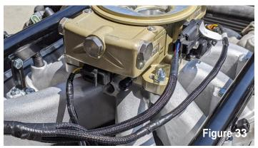
**IAC:** This harness connects to the idle air control motor that is mounted on the rear of the throttle body.
