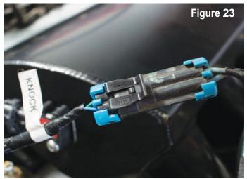
**KNOCK:** This sub-harness attaches to the Knock Sensor connector located on the side of the block on the LS2, LS3, and on the back of the block on the LS1, LS6.
