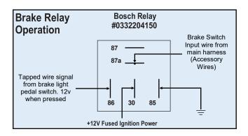
**Brake Switch Relay:** For use on brake pedal circuit if switch supplies 12 volts when the brakes are activated. ECU requires 12 volts when brakes are not activated. Wire as shown to achieve this.
