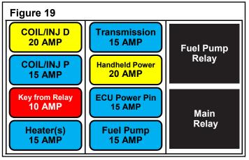
**Fuse Box:** Above is a graphic showing the location of the various fuses in the supplied Fuse Box which is item 6 in Figure 17.
