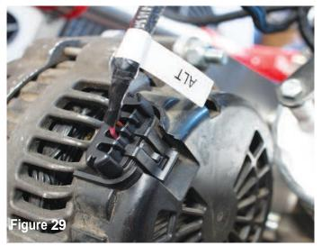
**ALT:** This wire directly connects to the alternator.
