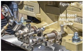
Idle Speed Adjustment Screw: Use only to adjust idle during IAC step settings. ECU must be put into correct settings mode before any adjustment is made on this screw or the ECU will continually adjust the IAC to maintain the previous idle speed setting. See Idle Screw Set TPS settings within hand held programming.
