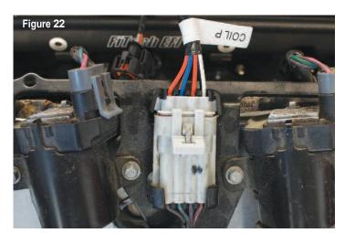
**Coil P:** The Coil P connector is connected to the existing connector on the passenger's side coil pack. **Note:** Coils and coil sub harnesses are not included in
