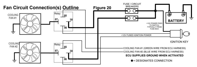
The Fan 1 (Green) and Fan 2 (Blue) wires are relay control wires – they should be connected to Pin 85 of the relay(s) that power(s) the fan(s). Pin 86 should be connected to a KEY Switched ignition source so that the fans turn off with the ignition key. Relay Pin 30 should be fuse or circuit breaker connected to the battery. Pin 87 should go to the cooling fans, and the other wire of the cooling fan should be grounded. Ensure the fan blows towards the engine. Each fan will require a relay.
