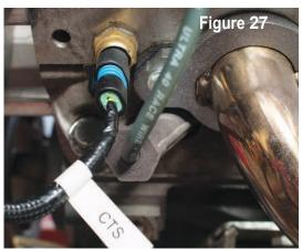
CTS: This wire connects to the coolant temperature sensor located in the front side of the driver's side cylinder head. The CTS is not provided in system.
