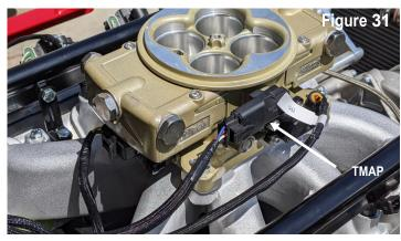
**TMAP:** Connects to the temperature/manifold absolute pressure (TMAP) sensor mounted on the side of throttle body. Sensor is pre-assembled onto throttle body from factory.
