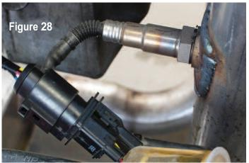
O2 Sensor Harness: There are two connectors on the main harness for the dual oxygen sensors. The connections are different types. The connection for the drivers side sensor allows the oxygen sensor to plug directly in. The connection for the passengers side is a 6-pin connector (yellow insert in black housing). This connection requires the use of the extension/adapter harness (shown right) that is included in system. Reference Figure 16 on page 8 for sensor installation instructions.
