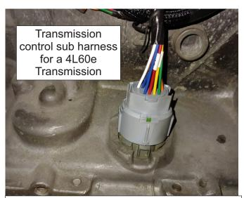
NOTE: The arrow on the transmission connector must be facing outward on the passenger side.
