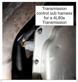
NOTE: The arrow on the transmission connector must be facing top side on the driver side.
