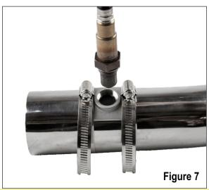
**WARNING:** Do not start the engine without the sensor cable connected to the throttle body and the EFI system is fully operational or damage will occur to the sensor.
