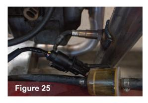
**TMAP**: Connects to the back of the manifold; Install with the bolt
