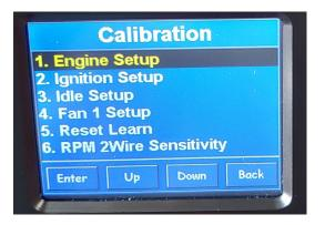
(Note: When changing values on the handheld controller, you must press the joystick button to SEND your info to the ECU. You will then see 'Sent to ECU Succeed' message which is a confirmation (Note: When changing values on the Handheld Controller, you must depress the joystick button to SEND your info to the ECU. You will then see 'Sent to ECU Succeed' message which is a confirmation
