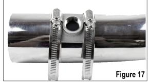
**H.** Install the sensor into the bung, see figure 18. Apply a small about of anti-seize on the threads of the O<sub>2</sub> sensor. Be very careful not to get any anti-seize on the tip of the sensor itself because it will cause it to prematurely fail.
