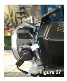
TPS: Throttle Position sensor: on throttle body
