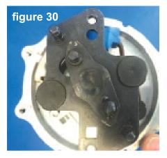
7) Put the engine at about 10 degrees BTDC, and move the distributor with the cap off to see that a tooth on the trigger lines up with the pickup sensor.
