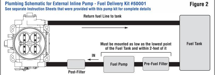
**Note:** Before starting any installation, disconnect the ground connection on the battery. Be very careful when disconnecting any fuel lines to let the fuel drain into a re-
