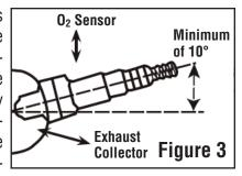
haust leak can create detonation and possible severe engine damage. Incorrect installation of the sensor, exhaust leaks, and any resulting damage is not covered by the FiTech manufacturer's warranty. Make sure your exhaust is leak-free. This is very important.
